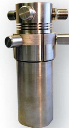
M7800 pressure cell U.S. Patent: 8,813,542
